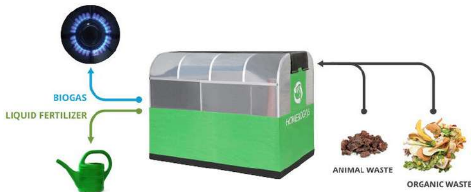
Figure 3. Scheme of the composting process and accumulation of residual gases
