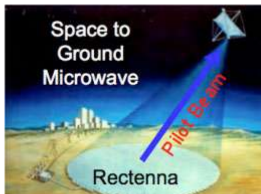
Figure 3. A laser pilot beam guides the microwave power transmission to a rectenna
