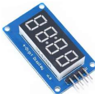
Figura 5: Modul LED Display Ceas TM1637 [5]
